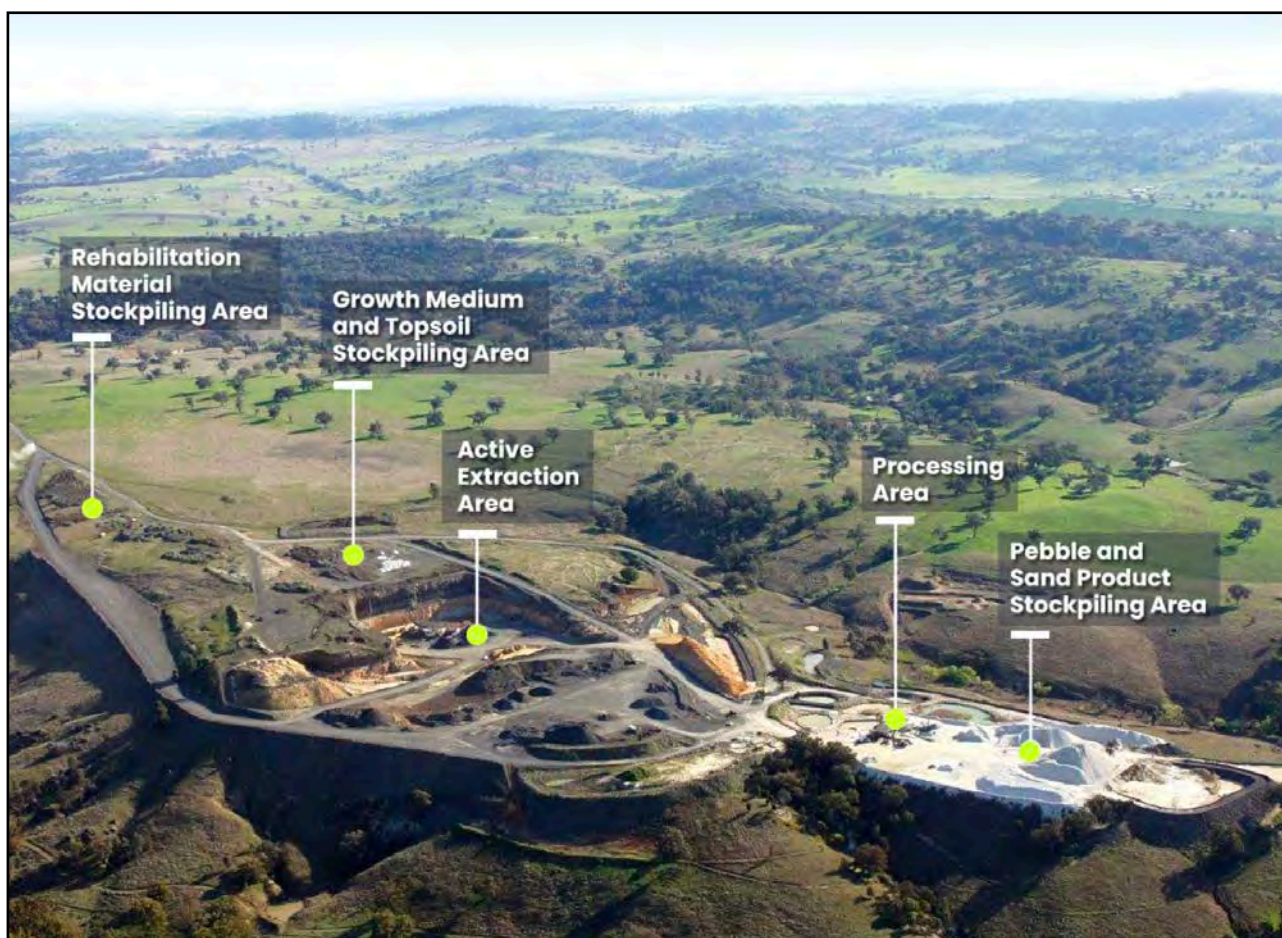
PHOTOGRAPH 2: Drone photography from north-east of quarry over existing quarry stockpiles, active extraction area, and processing areas
